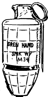
M34, WP smoke hand grenade (standard color and markings). Color/markings: light green, yellow band, red printing. Old markings: light gray, yellow band, yellow printing.
